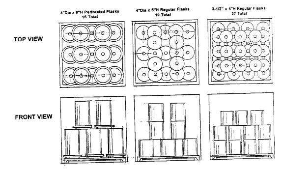
NOTE: THESE EXAMPLES SHOW CAPACITIES FOR OUR W18 FURNACE. THE SAME PRINCIPLES APPLY FOR ANY BURNOUT FURNACE.
